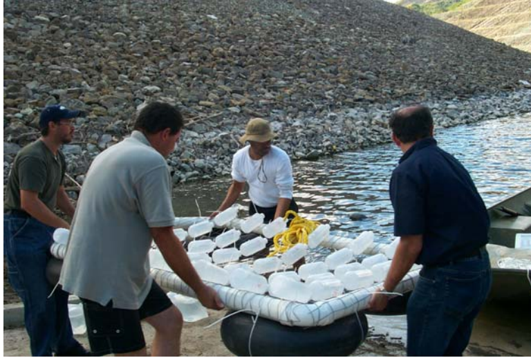
Figure 9. Deployment of the Matlock periphytometer at the Cerrillos lake (2/4/04).
