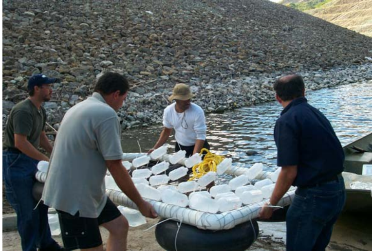
Figure 3-1. Deployment of the Matlock periphytometer at the Cerrillos lake.
