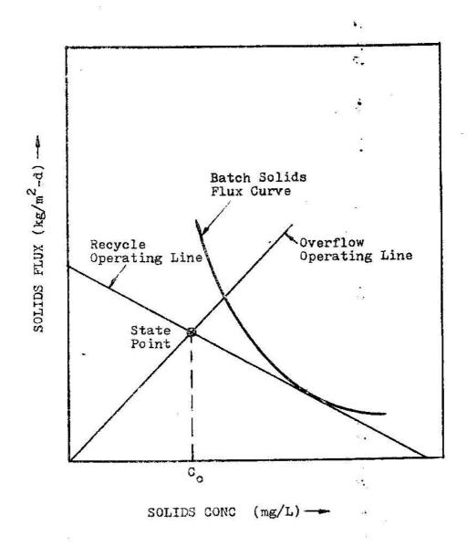
FIGURE 2 TYPICAL BATCH SOLIDS FLUX CURVE AND OPERATING LINES
